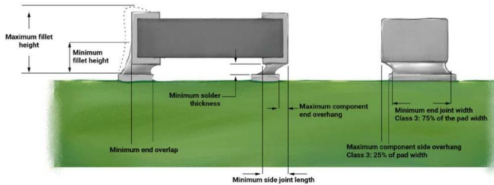
**Figure 5 : DFA criteria for surface-mount passives.**
