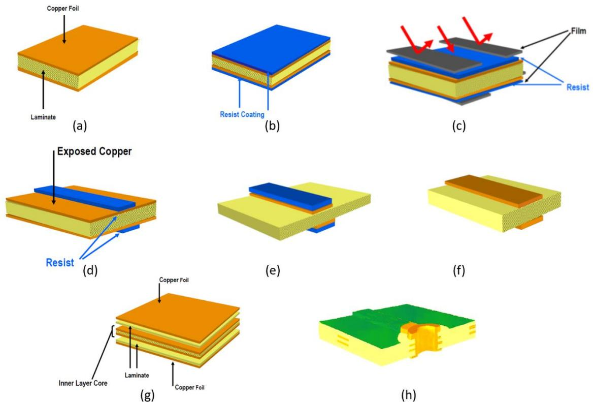
**Figure 4 : (a) inner core (b) addition of photoresist (c) addition of artwork film and exposure to UV radiation (d) chemical developer removes resist from areas not polymerised by light (e) etch away copper not covered by resist (f) removal of resist (g) sequential lamination of outer layers (h) addition of soldermask.**
