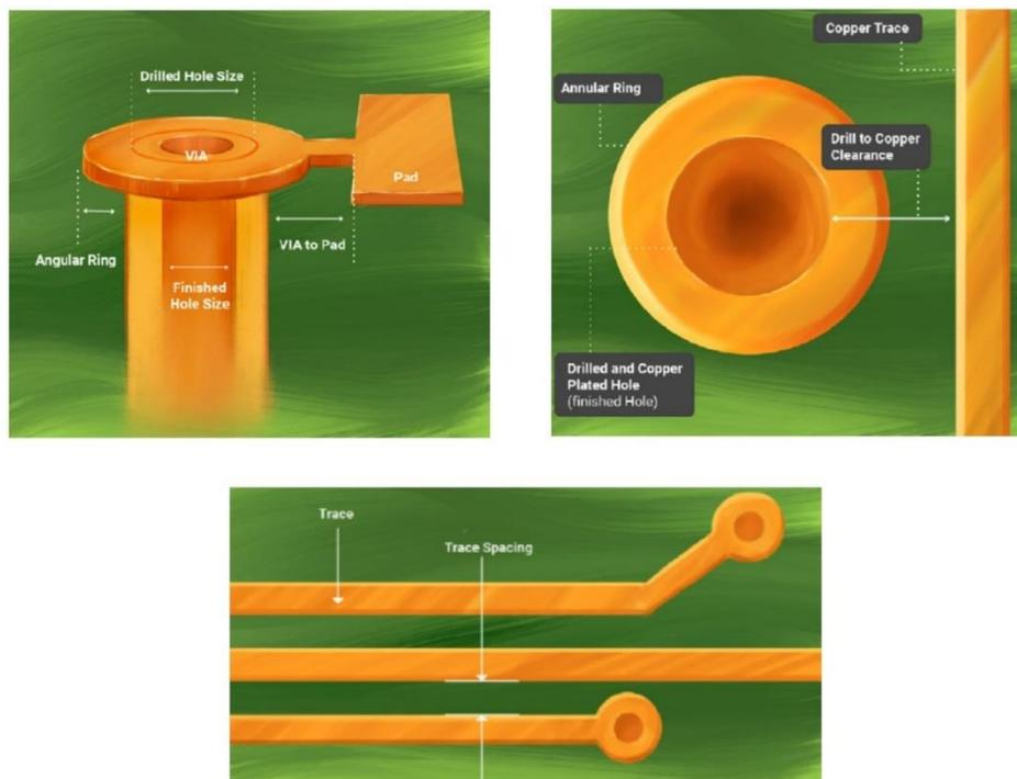
**Figure 2 : Illustrations of PCB DFM checks.**
