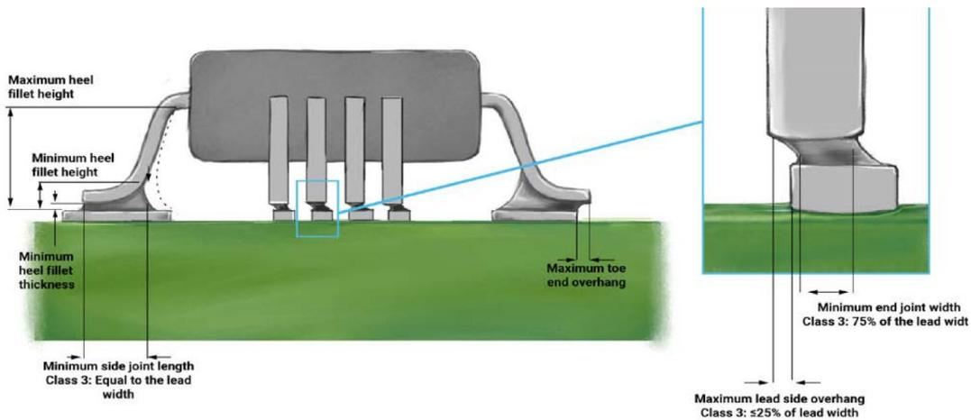
**Figure 6 : DFA criteria for surface-mount, gull-wing semiconductors.**
