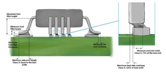
Figure 6 : DFA criteria for surface-mount, gulled-wing semiconductors.
