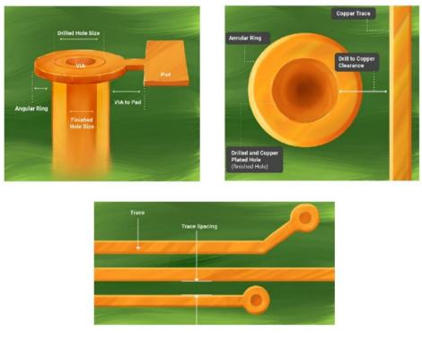
Figure 2 : Illustrations of PCB DFM checks.
