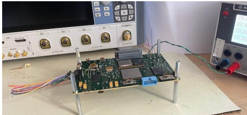
Figure 5 : Typical EM Testing in a Lab. Using Exposed Hardware.
